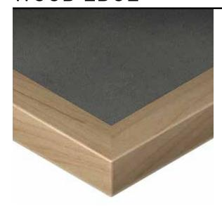
Edge table tops in Red Oak and Maple wood options. Our tops are manufactured with a choice of either a horizontal grade laminate or veneer top surface as chosen by you, and bonded to a 45-pound high-density particle board with a phenolic backing sheet. All wood edges are available to match our UV house finishes, standard with a catalyzed conversion satin sheen finish. Custom finishes are also available on request.
