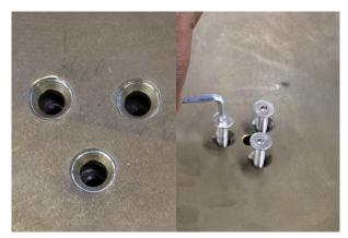
PLACE BOLTS IN THE ALIGNED HOLES AND USE THE ALLEN KEY TO TIGHTEN THE BASE TO THE COLUMN. (REPEAT FOR EACH COLUMN)
