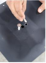
ATTACH THE TOP PLATE TO THE COLUMN USING TWO BOLTS AND FINGER TIGHTEN THEM.
