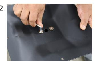
USE THE ALLEN KEY TO FIRMLY TIGHTEN TOP PLATE TO COLUMN
