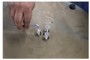
PLACE BOLTS IN THE ALIGNED HOLES AND USE THE ALLEN KEY TO TIGHTEN THE BASE TO THE COLUMN
