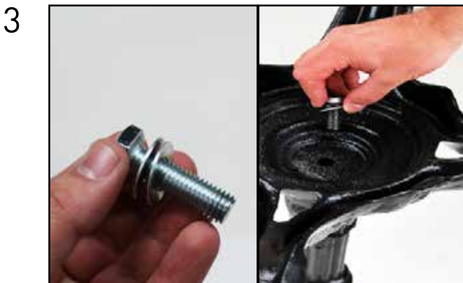
USING THE TWO FLAT WASHERS AND A BOLT FINGER TIGHTEN THE BOLT UNTIL SNUG.
